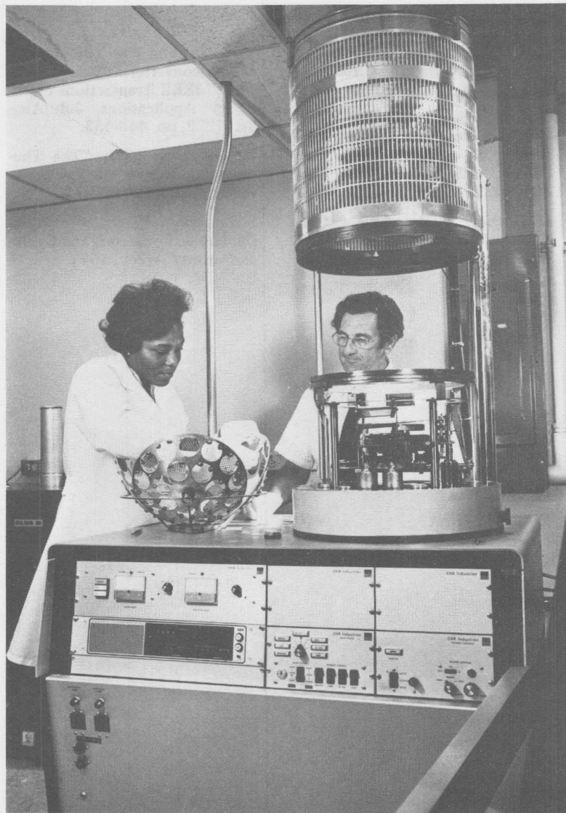
A vacuum evaporator used during the epitaxial growth of SCR junctions.
