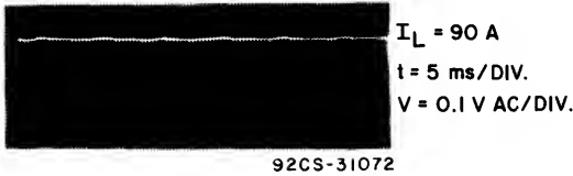
Fig. 171 - Hum performance of 900-watt converter system.
