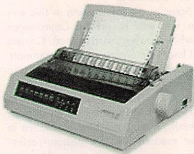
DOT-MATRIX PRINTERS are the only type of impact printers widely sold today.
