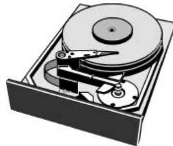
fig. 21: Hard disk, interior
