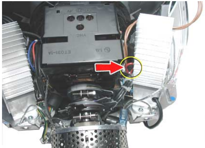
Voltage Jumper Location
