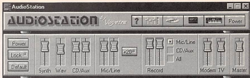
Fig. 5. If the sound board does not have a master volume control, check the board's "mixer" applet and make sure that the master volume is set properly.
