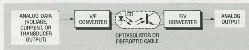
FIG. 10—ANALOG DATA CAN BE OPTICALLY COUPLED using two IC's, one as a V/F converter, the other as an F/V converter.
