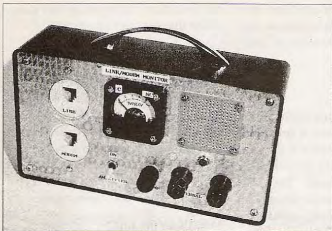
Photo A. Built-in voltmeter and speaker amplifier let you monitor the status of the phone line as well as hear what is on it.
