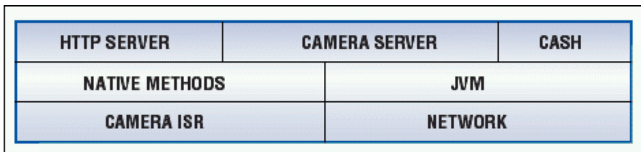
Figure 3. TINI streaming camera software supports both low-level and high-level protocols.
