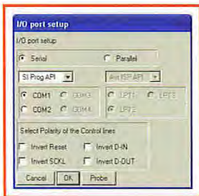
Figure 4. The correct settings must be configured very carefully in PonyProg before the microcontroller is programmed.
