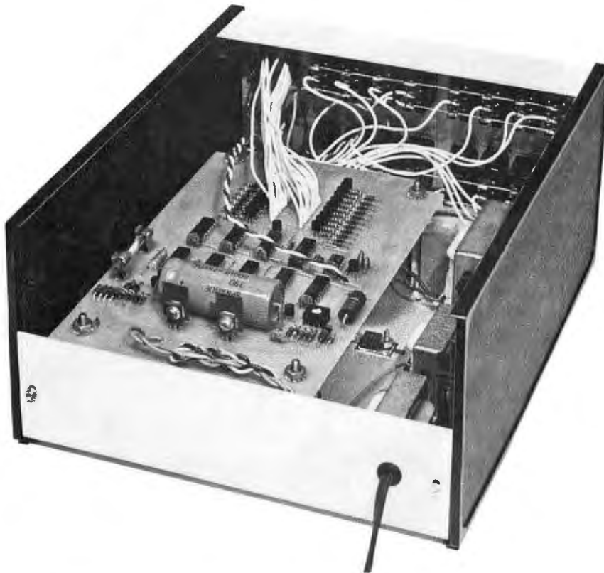
The 5-volt supply is mounted under the pc board. With a little care, as shown here, a very professional look can be attained.
