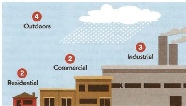
FIGURE 2. Pollution degrees describe indoor and outdoor environments. Artwork by Melinda Vaughan, National Instruments.
