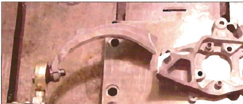
After 2.5 million cycles, the parts were tested to destruction at maximum loading, with the first failure occurring after an additional 2,481 cycles.
