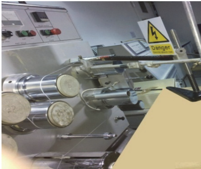
Fig. 4. Piezoelectric polyvinylidene fluoride (PVDF) filament production via a continuous process using a melt extruder
