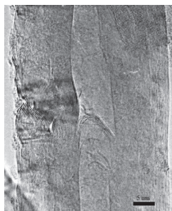
Fig. 4. HRTEM image of carbon nanotube prepared using catalyst with 3.5% iron (Wang et al., 2005a)
