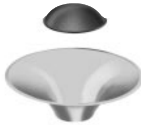
Bonding Dust Cap to Cone
