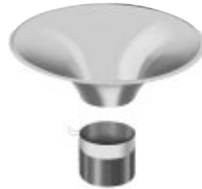
Bonding Lead Wires to Cone
