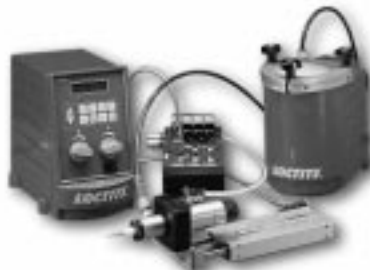
System shown includes 0.5 liter reservoir and stationary valve.
