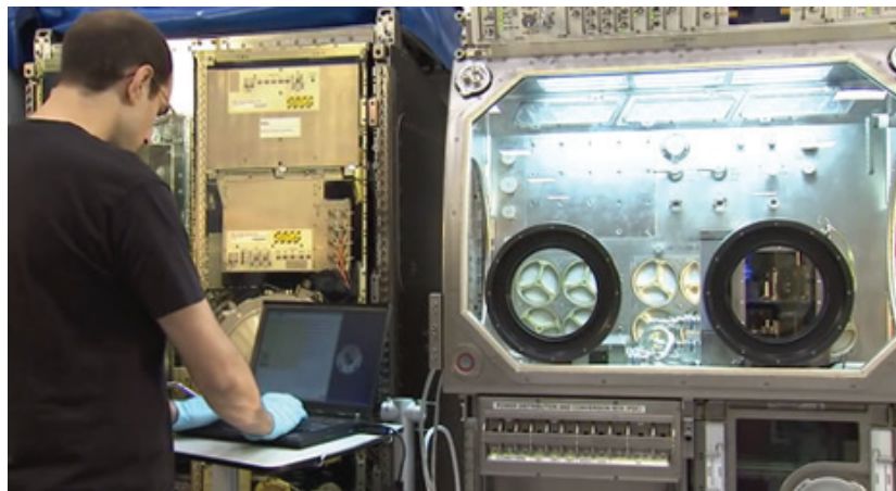
The 3D printer will operate inside the Microgravity Science Glovebox, a rack that provides a level of containment and filtration.
