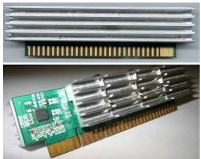
Figure 12 Heatsinks attached to multiple devices
