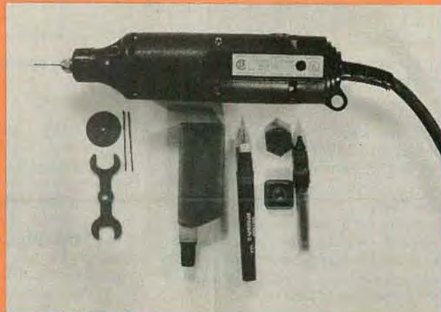
FIG. 1—TINTED SHELLAC, a Rapidograph or similar drafting pen, a high-speed rotary drill, and drill bits are the only tools you need to make high-quality PC boards.
