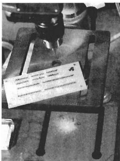
FIG. 5—PERFORATED CIRCUIT BOARD blank serves as a drill jig to obtain holes spaced in 0.10-inch increments.
