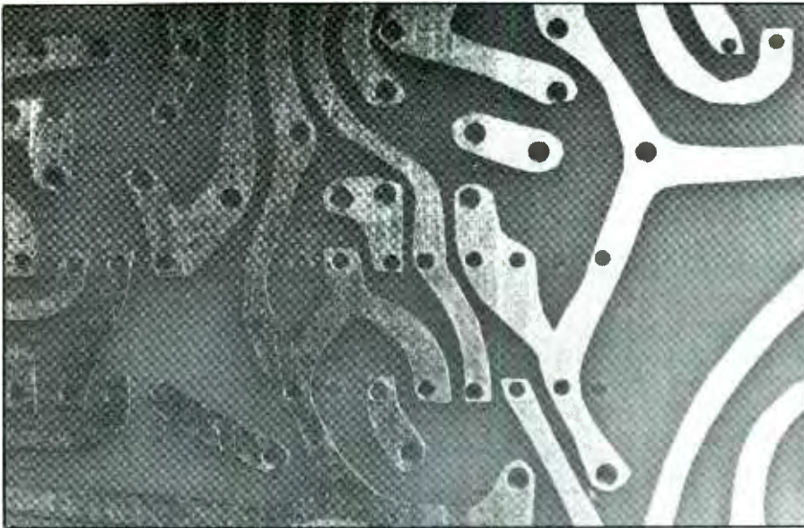
Fig. 5. After etching the pc blank and removing plastic-sheet "resist" and cleaning the blank, copper traces are sharply delineated from board substrate.
