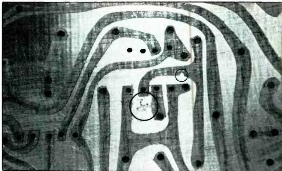
Fig. 4. After scoring around drawn trace pattern with sharp hobby knife and removing unwanted plastic sheeting, examination of result may show such potential problem areas like left-behind adhesive (inside large circle) and notches removed from traces (small circle).
