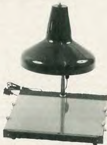
FIG 3—TO EXPOSE THE BOARD, place the sensitized blank and the photomask in a contact frame and place under a strong light source.
