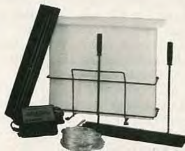
FIG. 5—TO AVOID TEDIOUS HAND agitation, you may want to use an automatic agitator like the one shown here.
