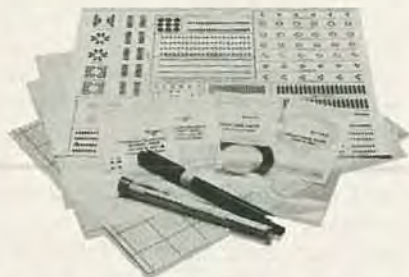
FIG. 6—YOUR ARTWORK can be transferred to a piece of Mylar film using drafting aids like these. The result is a positive photomask.
