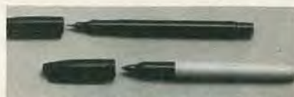
FIG. 7—PC ARTWORK CAN BE DRAWN directly on the copper blank using etch-resist pens. Lacquers and drafting aids can be used, too.
