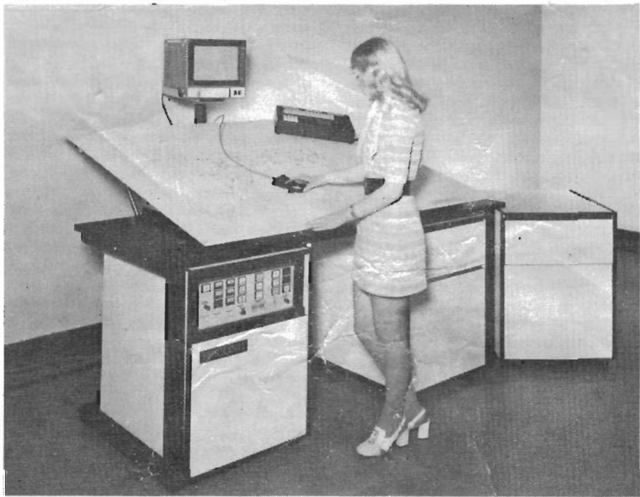
The Ferranti Feedraft used to automatically generate p.c. masters, i.e. masks and other drawings.
