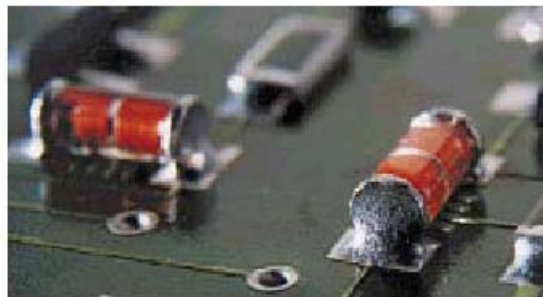
Cylindrical end cap terminations (MELF) (unit: mm)
