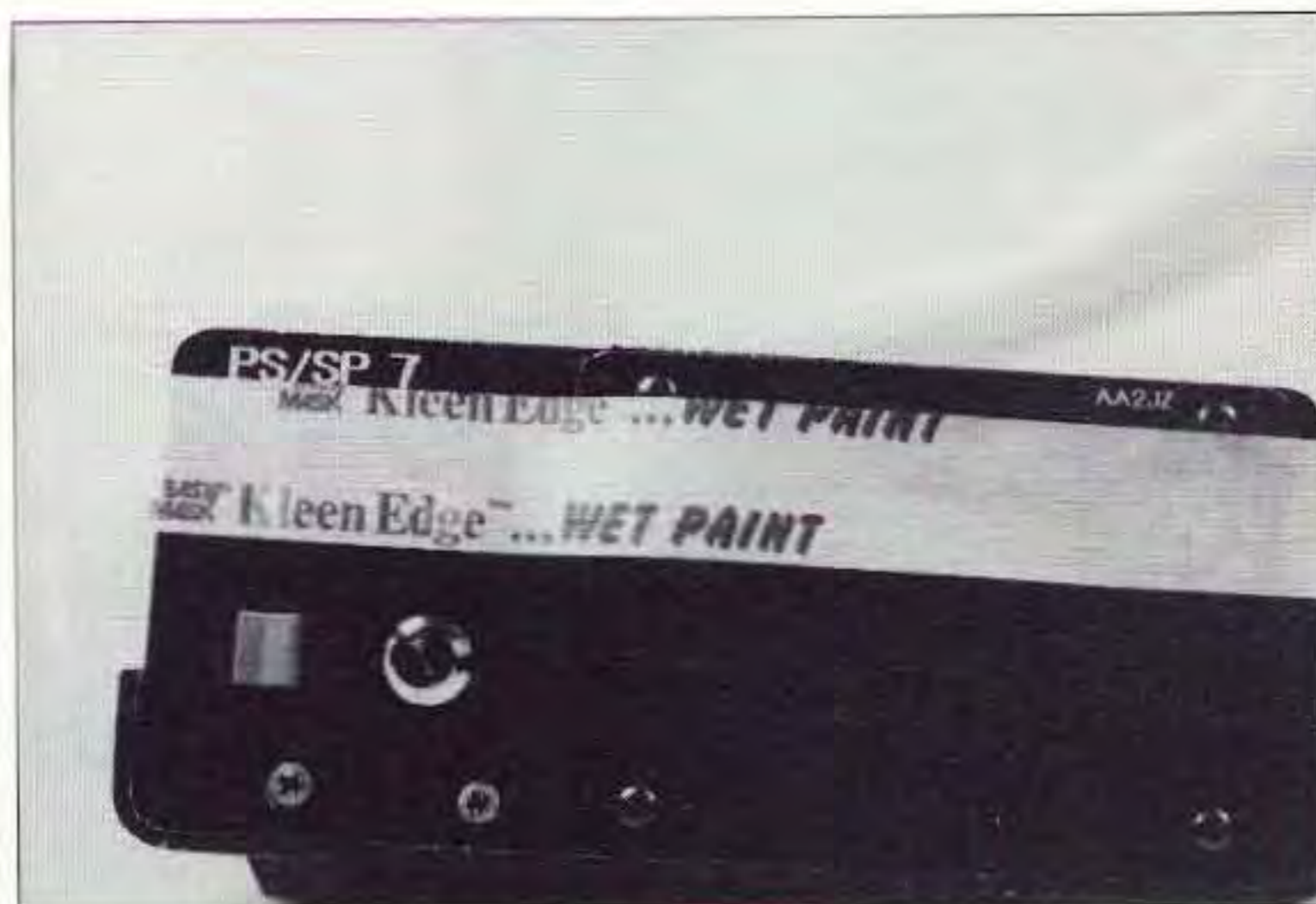
Photo C. Painter's tape is used to guide lettering into perfect alignment.
