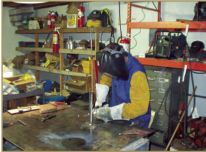
Willy the Welder added some extra protection to the welding glove on his left hand using a reflective pad. Photo courtesy of Steven Kirk Nelson and Pete Maxham.
