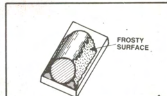
Figure 16. A cold joint can be deceptive. The joint may look good in other respects, but the solder surface will have a frosty appearance (see accompanying picture). Reheating the joint usually fixes it.
