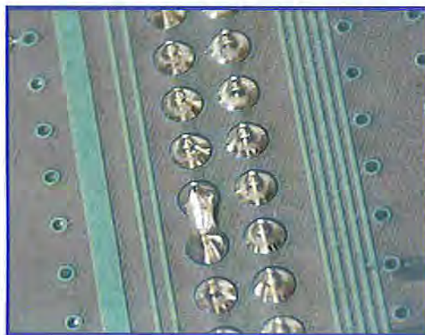
Figure 2. The formation of solder bridges can be avoided by the use of an inert atmosphere.
