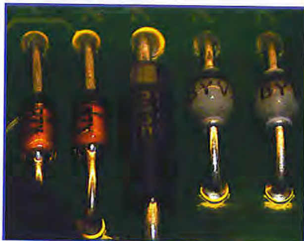
Figure 4. Because of the lack of lead, the shape of the joint is different.
