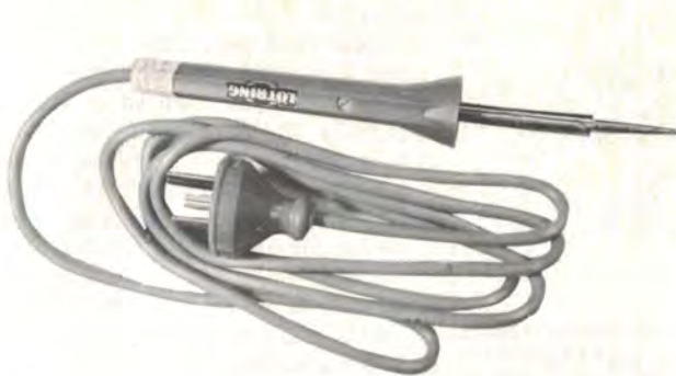
Figure 3. A popular continuous heat general purpose soldering iron, from Lotring. It has a heating element in the barrel and a tapered solid copper bit fits inside this, secured by a small grub screw at the end of the barrel. You can make your own bits for this sort of iron from copper rod.
