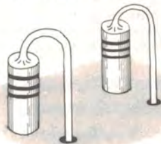
Figure 36. Whilst axial lead components (i.e. resistors) are generally mounted horizontally on a pc board, they are sometimes mounted vertically. Leave a millimetre or so clearance between the bottom end and the board.
