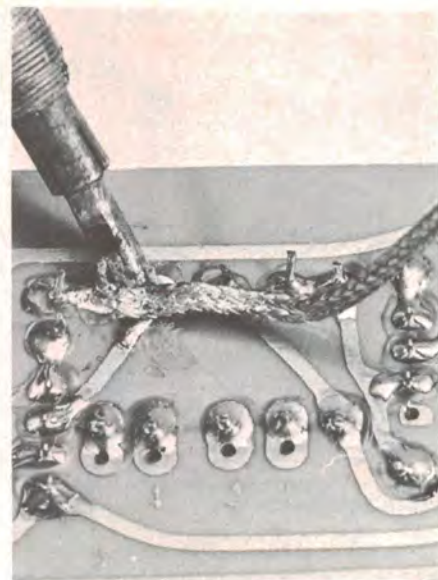
Figure 37. How to use desoldering wick. Lay it over the joint and apply the iron tip to the braid, using a little pressure. When the solder is drawn into the braid, remove the iron and the braid.
