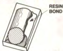
Figure 24. A resin bond. There may be no electrical contact at all. It can be cured by reheating the joint.
