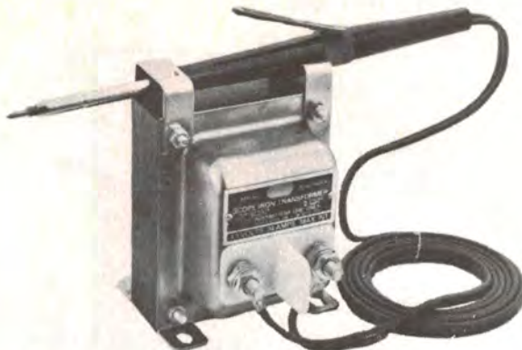
Figure 4. A quick-heat iron, Scope Lab's 'Mini Scope'. It operates from a 3 V/30 A transformer and is rated at 20-75 watts. Pressing the bar puts a carbon element against the tip, rapidly heating the element and the tip. This sort of iron is very useful for desoldering applications using solder 'wick'.
