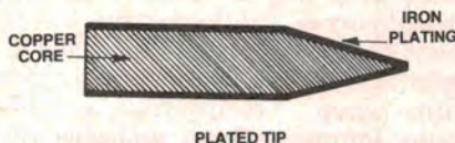
Figure 10. Plated bits last longer because they do not oxidise as rapidly as unplated bits. They are usually iron-plated.
