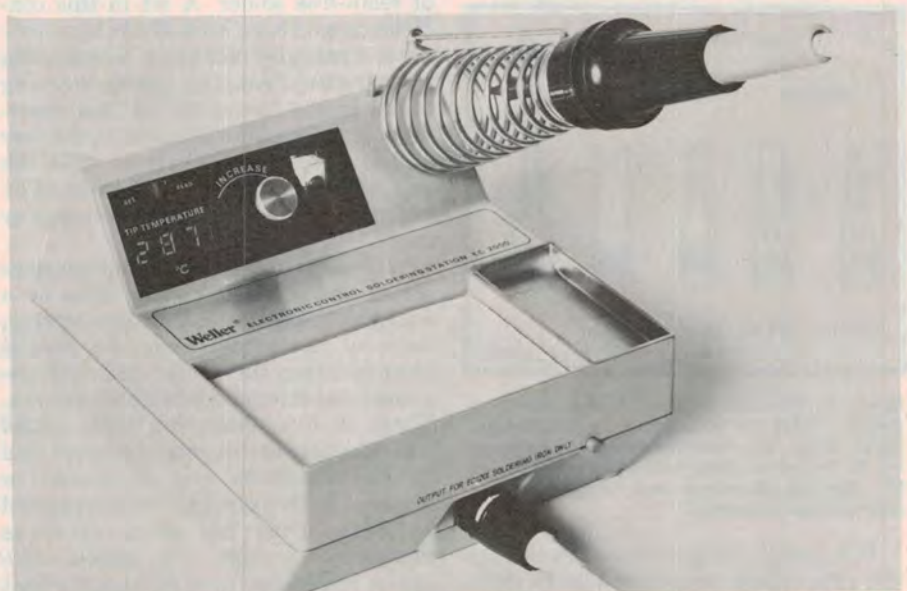
Figure 7. This iron, Weller's model EC2000D, employs a temperature sensor in the tip and electronic control of the power to the heating element to maintain the tip temperature within very close limits. The desired temperature is set by a knob and displayed in the three-digit readout.
