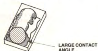
Figure 23. Too little heat. The solder forms a large contact angle with the surface and can be pried loose.
