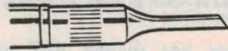
Figure 8. A typical replaceable soldering iron bit. This one screws onto the end of the iron barrel, and the cylindrical tip has a 'flat' on the end at an angle of about 60° to the axis.
