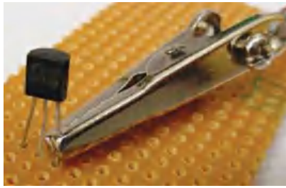
Fig. 3: A crocodile clip holding the heat-sink in place
