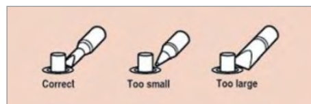
Fig. 1: Selecting the right soldering tip
