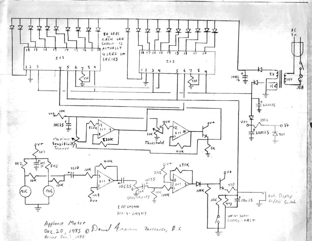
The applause meter is intended to help judge events by the level of sound generated by applause. The unit is to be hung from the stage ceiling and to be plugged into normal 120 Volt AC power. The remote unit is mounted in the DJ booth.
