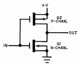
during the switching transition and this is very low. The output is then at the +V level. When the input goes high, QI turns on and Q2 turns off. Again only switching current flows and the output is virtually at ground. If the load is another MOS circuit, the latter will have a very high input resistance and require very little current. Only voltages are being switched. You can also guess that the actual value of +V is relatively unimportant so a well-regulated supply is not needed.
