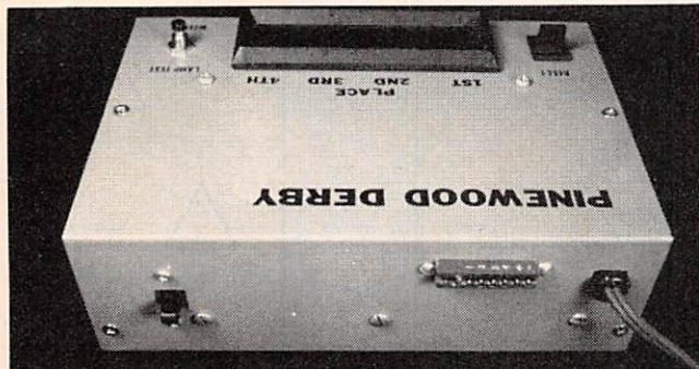
The view of the back panel shows the power cord with strain-relief, the power supply on/off switch (S51) and a ribbon cable connector that the author used. That connector interconnects the external photocell transistors on their printed-circuit board with the internal circuitry of the Scoreboard. Any connector will do, or you may elect to hard wire the ribbon cable directly to the Scoreboard eliminating the need for a connector. Exactly how you do it is up to you!
