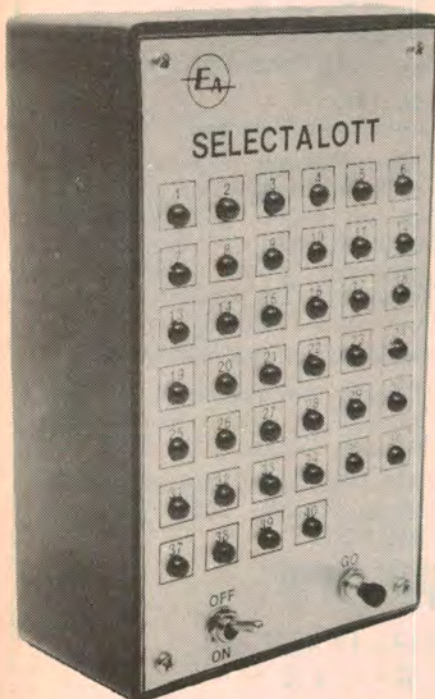
Selecting Lotto numbers is easy — just switch on and press the GO button.
