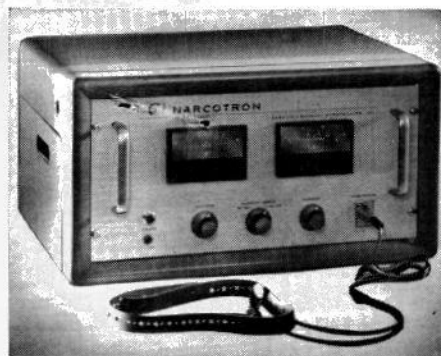
Carolina Medical Electronics, Inc. A typical commercial electrical anesthesia device that uses 700-cycle sine waves.
