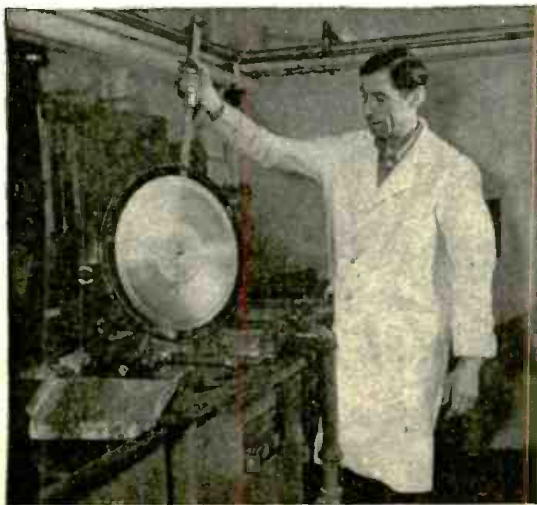
8 —CHROMIUM PLATING—And that isn't all. A technician dips the disk into a chromium bath. It comes out chromium-plated, after which it goes to a drying oven. A final smoothing and aligning operation follows.
