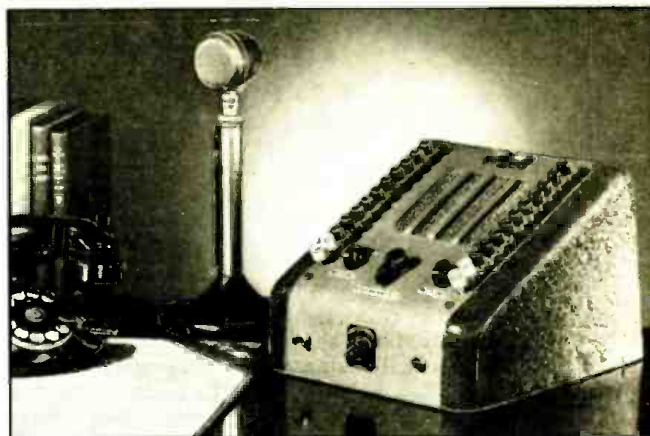
Operadio system TES will work in schools of 20 rooms or less. Outfit includes master control, unit amplifiers, 10 speakers with cabinets, mike & stand. Not included is phone at left, which may be used for calling up blonde.
