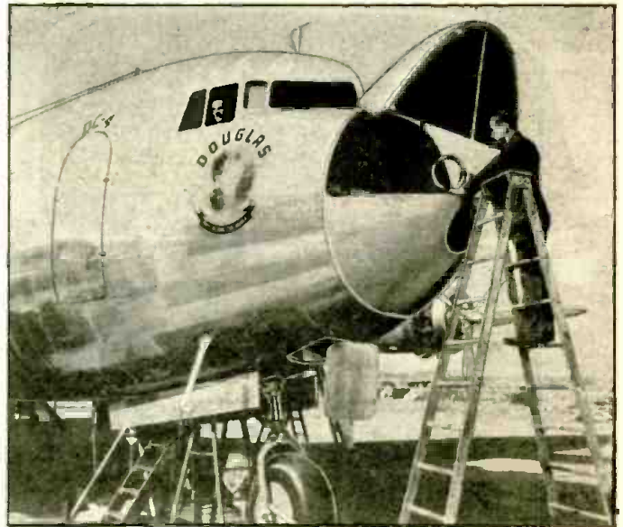
E. A. Post, communications engineer of the United Air Lines Transport Corporation, inspects the DC-4's direction-finding loop antenna by means of which the celebrated 30-ton air giant ascertains its exact position relative to beacon stations. Two additional receiving antennas are installed beneath the ship and its pilot's voice is flashed from a slender wire stretching above the 42-passenger cabin.
