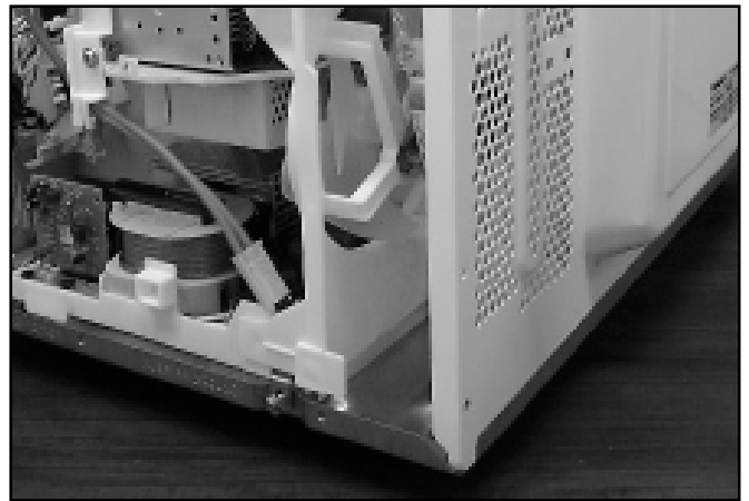
5. Remove screw and slide orifice toward you, then lift up and out.
