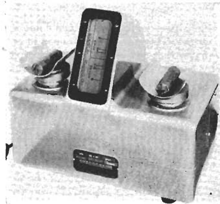
Fig. 8. Shadowgraph coin-counting scale is basically the same device shown in Fig. 7. Roll of coins is balanced against an exact count of coins in another roll. Over or underweight condition is indicated by projecting a line on translucent scale.
