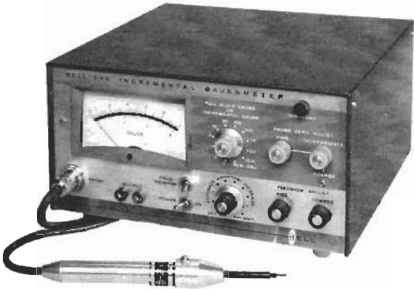
Fig. 3. Sensitive gaussmeter by Bell measures small fields.
