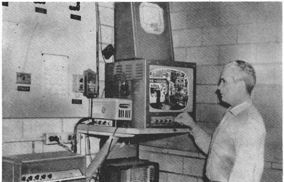
Shift foreman at Esso Research & Engineering Co. pilot plant at Bayway, N. J., checks safety of workmen on job at unit 300 feet away via General Precision Labs closed-circuit TV system.
