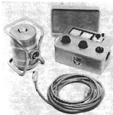
Fig. 6. Portable x-ray apparatus of this type is common in industrial radiography.
