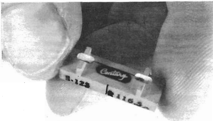
Fig. 3. Typical commercial silicon strain gage in its holder.
