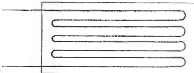
Fig. 1. Wire in a strain gage is looped back and forth in order to produce desired resistance change when it is bent.
