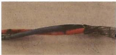
Typical FireWire cable with an aluminized polyester shield after 100,000 cycles of rolling flex on a 50 mm bend radius. Insulation and conductor damage appear where shields have cracked.
