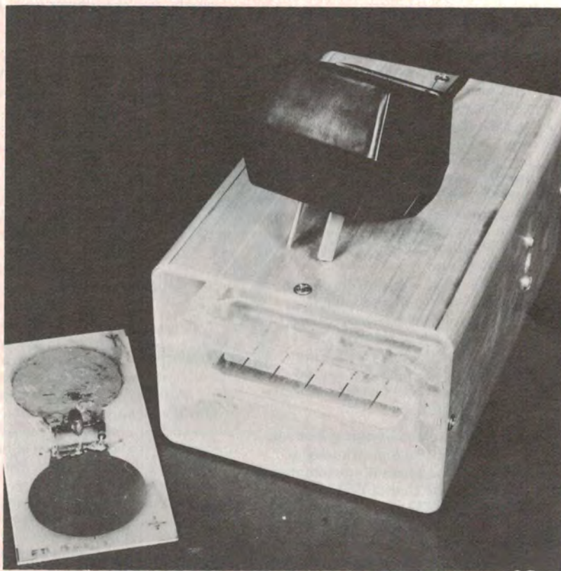
Our unit can be powered from 12 Vdc or a plug pack. The blinker testing device is at left.
