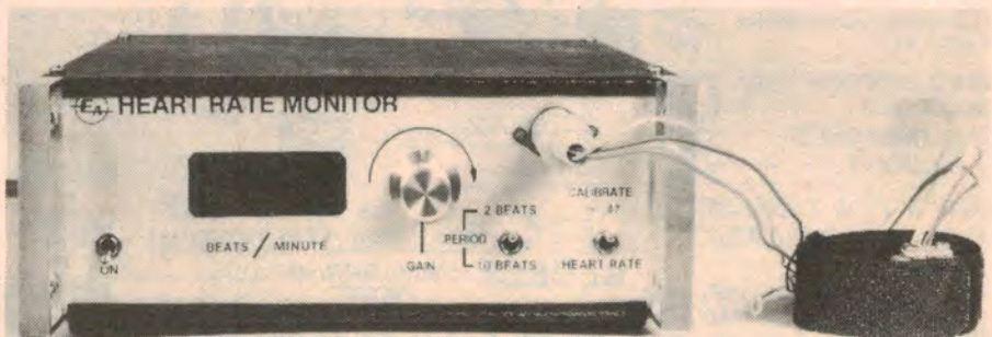
Pictured above is the Heart Rate Monitor together with the wrist-strap sensor. It can be used during any stationary exercise such as pedalling an exercise bike, as pictured at top left (Photo courtesy of "Vital" magazine).
