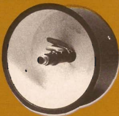
FIG. 6—INTERIOR VIEW of the top PVC cap. Rectifier D1 and capacitors C4, C5, and C6 are shown.
