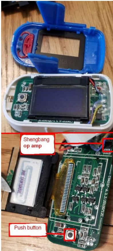
The pulse ox with the screen bezel removed, top, and with the LCD flipped up to reveal the numerous discrete components mounted to the PCB beneath it, bottom.
