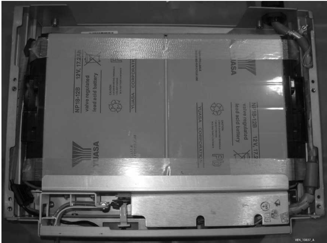
Figure 8-120. Four-hour battery cable routing
