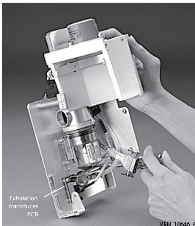
Figure 8-82. Replacing exhalation transducer PCB
