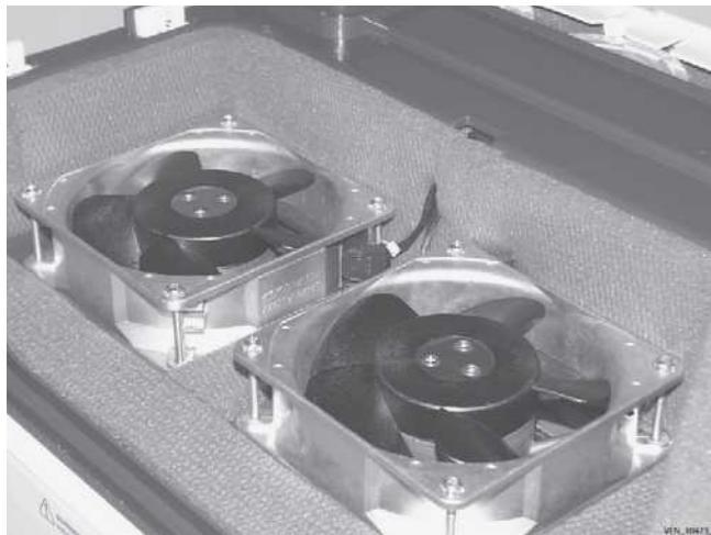
Figure 8-94. Fans installed in compressor
