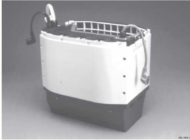
Figure 8-93. Top cover removed from compressor
