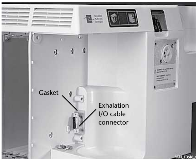
Figure 8-84. Removing BDU housing
