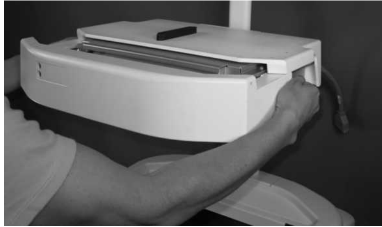
Figure 8-118. Removing BPS bezel
