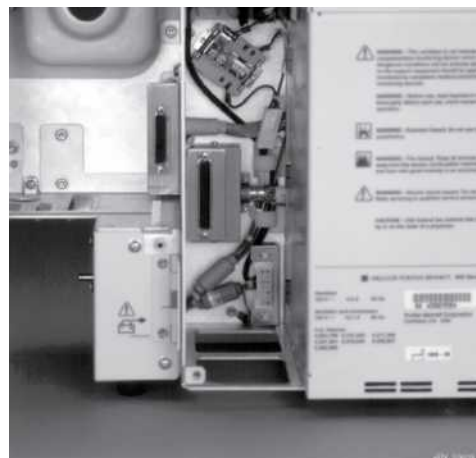
Figure 8-54. Replacing humidifier receptacle
