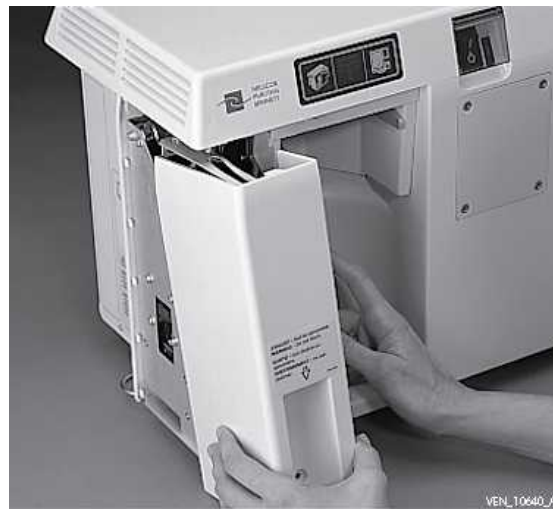
Figure 8-75. Removing exhalation module cover
