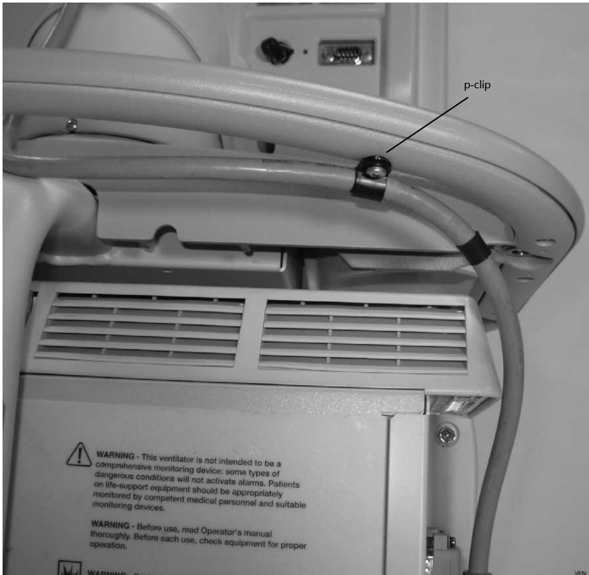
Figure 8-4. P-clip and GUI cable installed on Puritan Bennett 800 Series Ventilator Pole Cart
