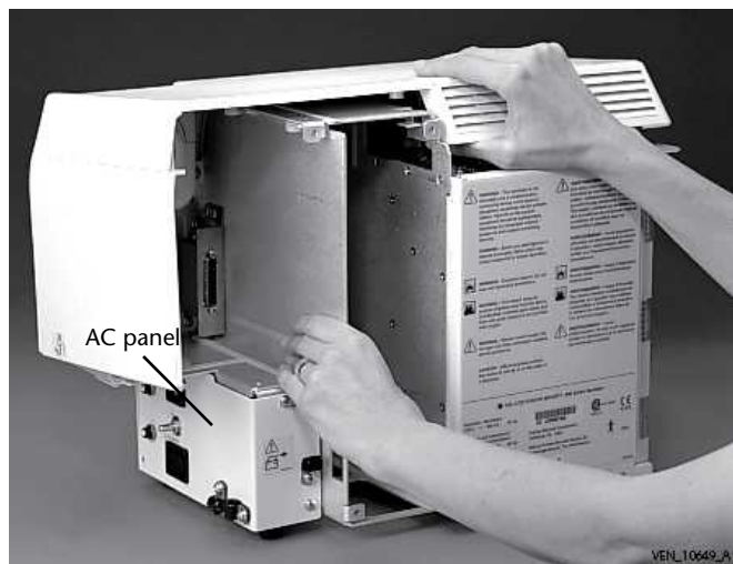
Figure 8-84. Removing BDU housing
