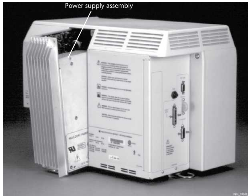
Figure 8-51. Replacing power supply assembly
