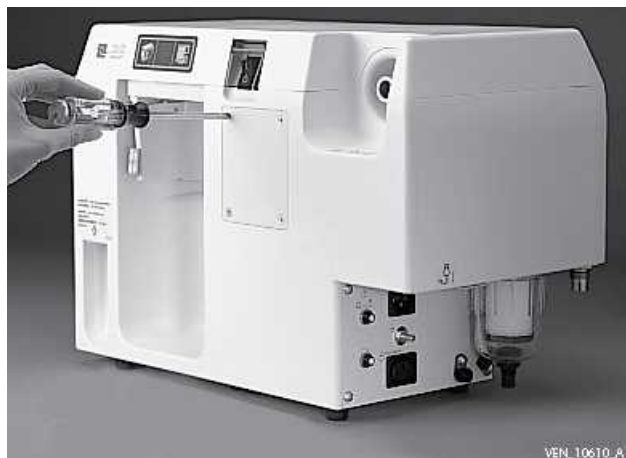
Figure 8-54. Replacing humidifier receptacle
