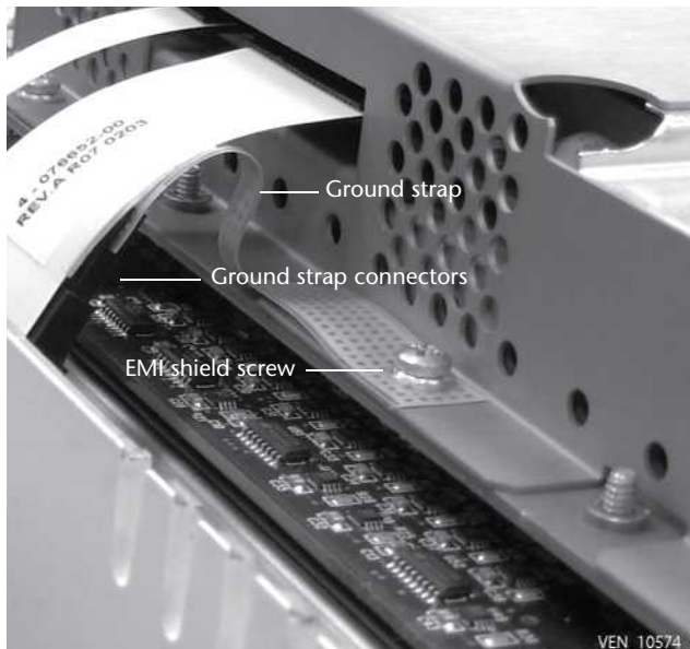
Figure 8-21. How to attach the grounding strap to the EMI shield
