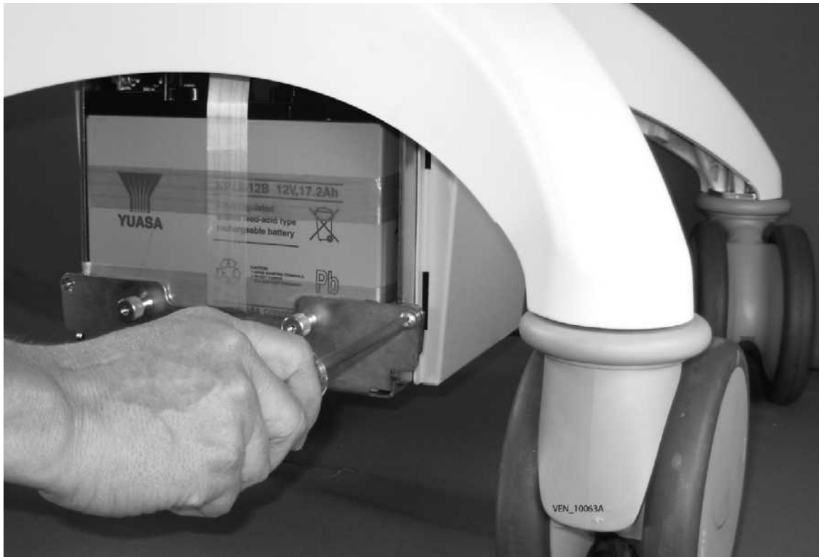
Figure 8-127. Securing Phillips screws on Puritan Bennett 800 Series Ventilator Pole Cart battery carrier (four-hour battery shown)
