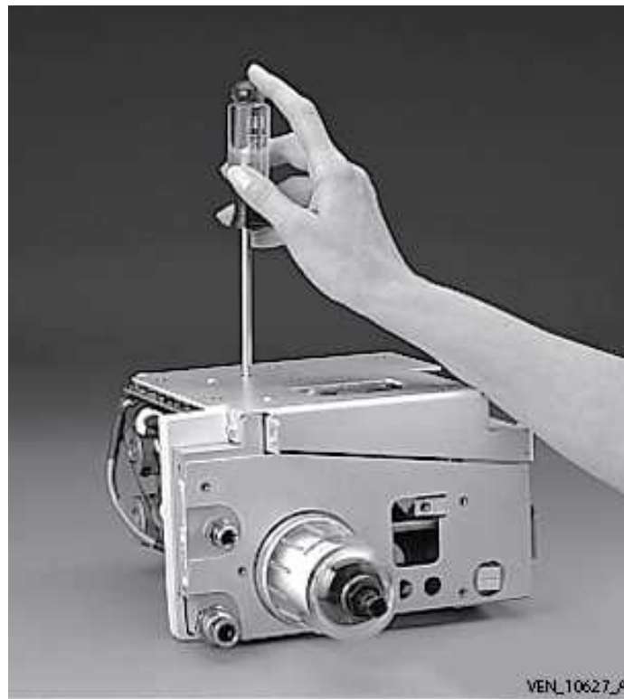
Figure 8-67. Removing inspiratory module right-side plate
