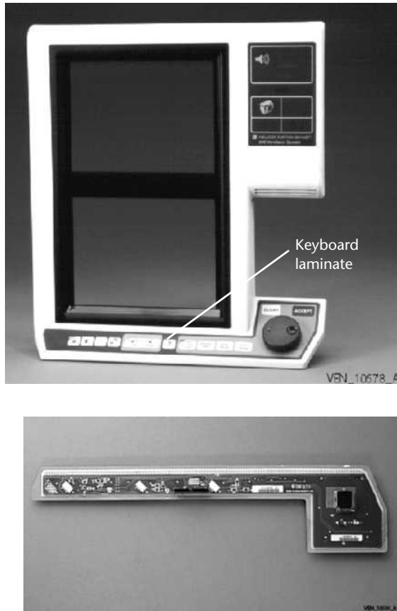
Figure 8-25. Replacing the 9.4-inch keyboard assembly
