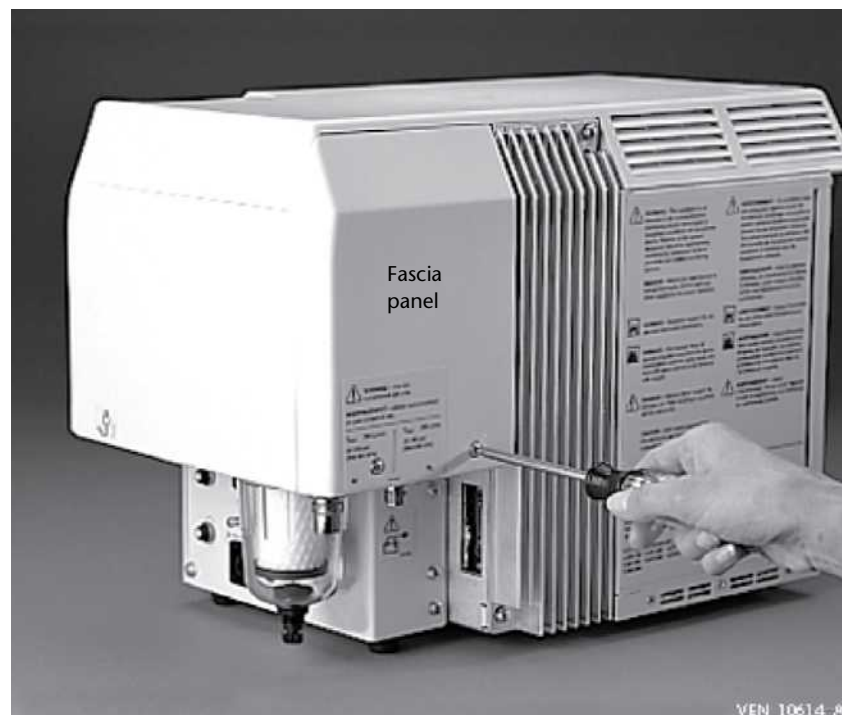
Figure 8-58. Removing inspiratory module fascia panel
