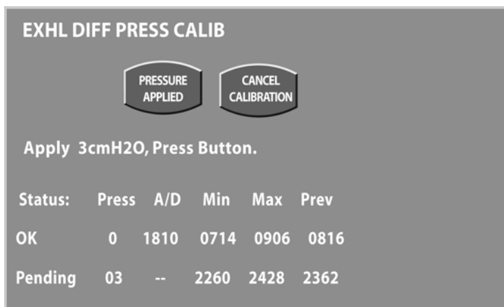
Figure 4.47 Exhalation Differential Pressure (Flow) screen #2
