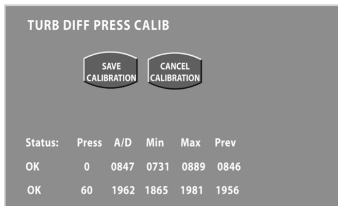
Figure 4.45 Turbine Pressure 60 cmH 2 O calibration screen #3
