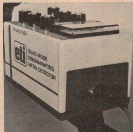
A view of the forward end of the case showing the two battery test pushbuttons and the DIN plug and socket connection to the search head. The Altek cabinet is two-tone grey plastic. The upper section is a lighter hue. Note the "GT" stripes!
